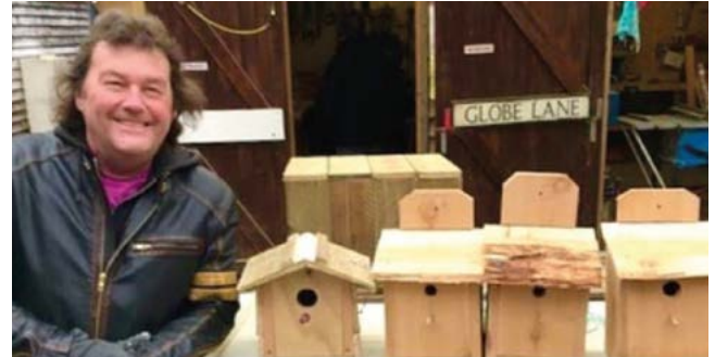
Above: Community 'Shedder' Tim with some bird boxes he has made in the past. The different-sized holes allow various birds to enter: 25mm for blue tits, 28mm for great tits, 32mm for house sparrows. A starling needs a 45mm hole
